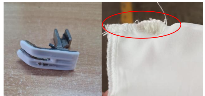
Fig. 8 Functional wear of the needle guide (bakelite) and its influence on sewing quality.
