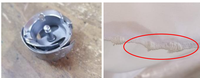
Fig. 7 Evidence of hook deterioration and its impact on the quality of the stitching.
