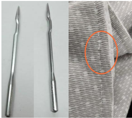
Fig. 6. Degradation cycle: new needle, worn needle, and fabric damaged by faulty stitching.
