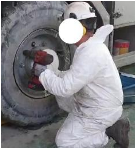
Fig. 6 Removing tire studs
