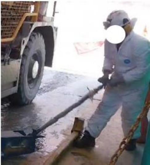
Fig. 5 25TN Hydraulic jack position.
