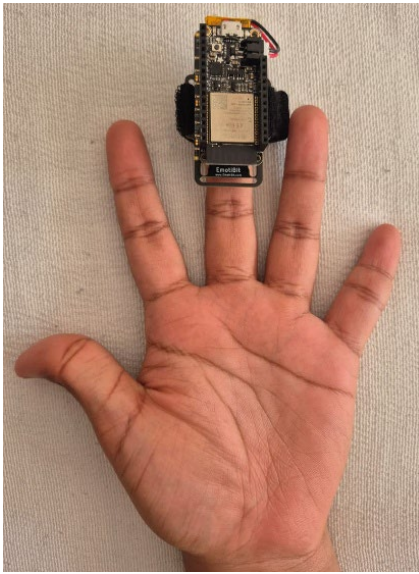
Fig. 2. Emotibit device for signal acquisition.
