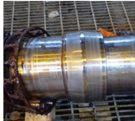
Fig. 11. Inner ring wear
