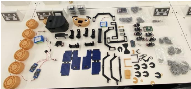
Fig. 2 - Component Parts for the ExoMy Rover Project after 3D Printing
