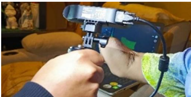
Fig. 1 High-precision digital acquisition of the residual limb geometry using the CR Ferret Pro 3D scanner to ensure anatomical socket fit.
