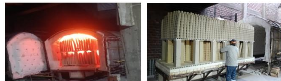
Fig. 5. Refractory crucibles in calcining area.
