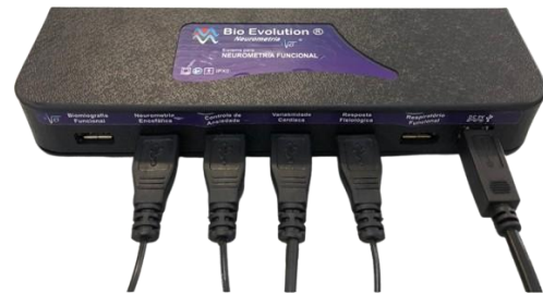
Fig. 2 Cabinet with channels for connecting the sensors
