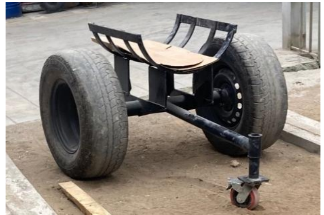
Fig. 4 Second pilot test for mold transport device
