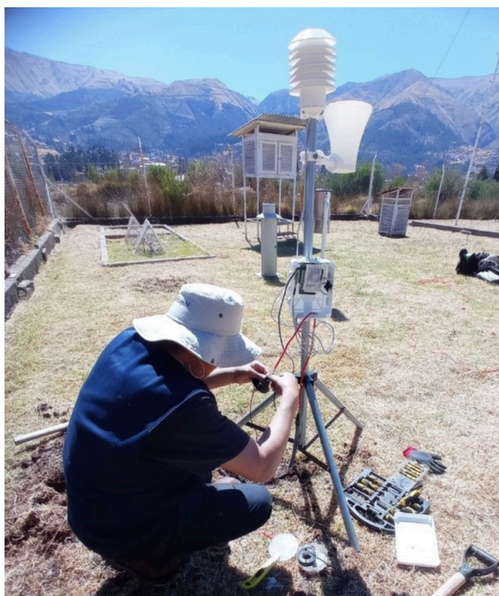
Fig. 2. State of the art 2: Semanhi weather station 3D-printed in PLA, installed in Cusco.
