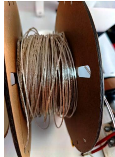
Fig. 6 PET filament with trapped air.
