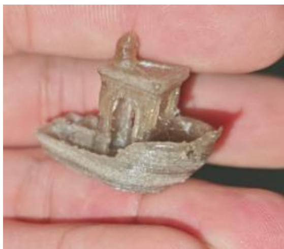
Fig. 8 Printing with PET filament "Benchy".
