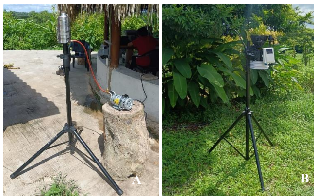
Figure 2. (A) non-viable cascade sampler TISCH Environmental®. (B) Weather station, Davis Vantage Pro®
