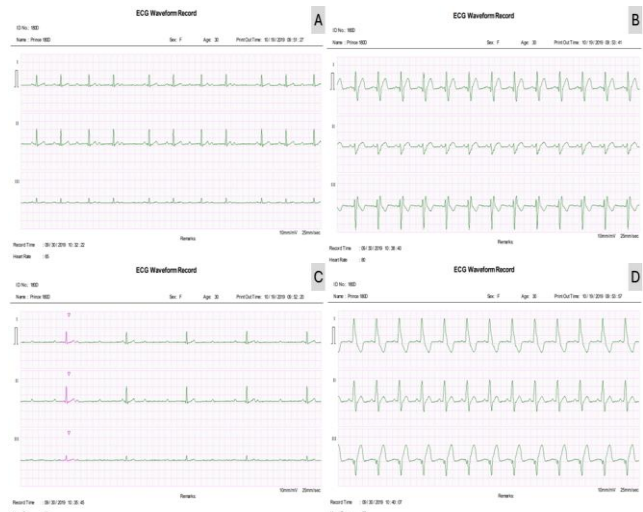
Fig. 4 Pathologies simulated on MECG 180D device for sensitivity purposes performed with the PS-2200 multi-parameter patient simulator
