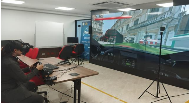
Fig. 3. Execution of the simulator using virtual reality glasses and video wall simultaneously.
