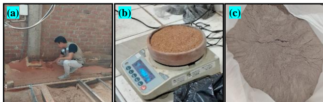
Fig. 2 Photographs of (a) pine sawdust collection; (b) weighing of pine sawdust for incineration; (c) pine ash (PA).
