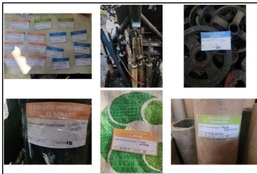
Fig. 6 Visual tagging system for 5s implementation
