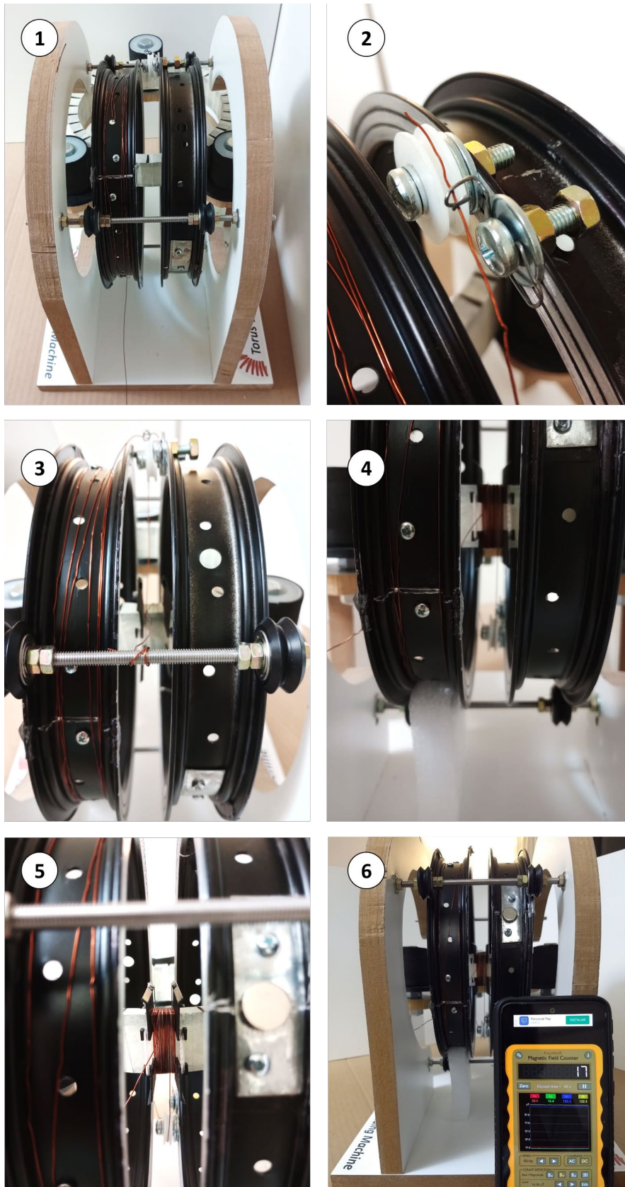
Fig. 5 Operation steps of the developed device to wind a slotless toroidal stator. 1) loading operation, 2) feeding the wire through the threader and small wheel, 3) holding the wire for the first couple of turns, 4) placing the friction brake, 5) winding the coil, 6) counting the number of turns.
