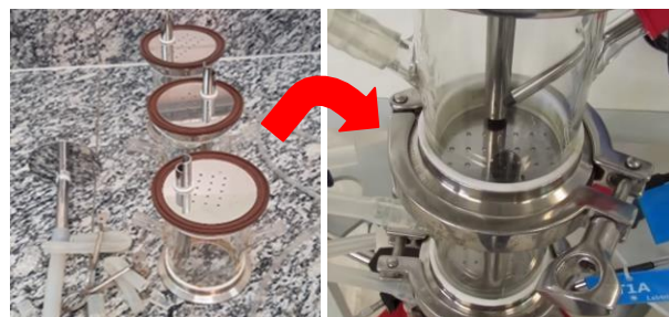
Fig. 12 Fourth experiment stages assembly
