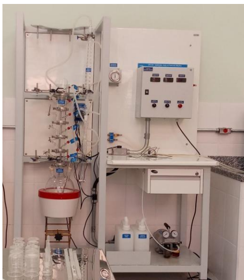
Fig. 2 Labtrix XP1520.3 distillation column
