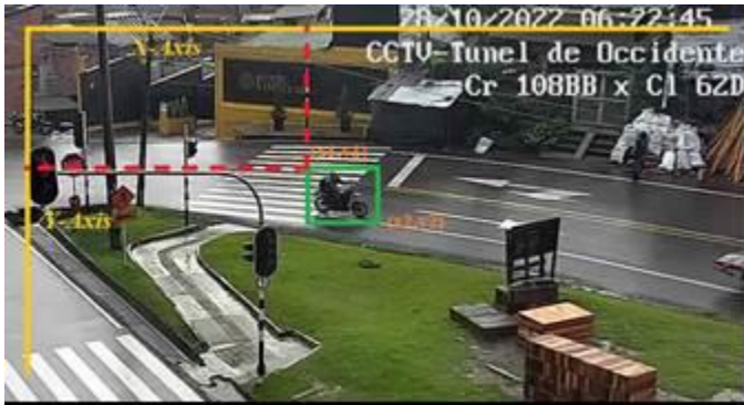
Fig. 1 Example of a selected ROI for an object of a specific class.
