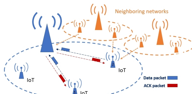
Fig. 1: A LPWA scenario with IoT devices where collisions among other IoT devices and interference from other networks requires to introduce novel access schemes.
