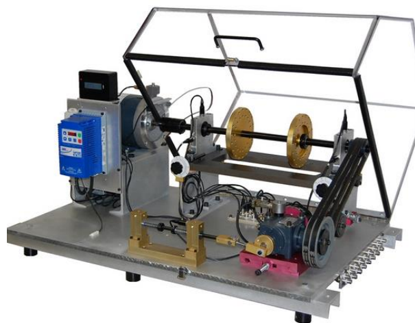
Fig. 6. Machinery Fault Simulator by SpectraQuest. This equipment can simulate typical faults such as imbalance and misalignment conditions. It also includes a variety of damaged components (damaged on purpose) such as bent shafts, ball bearings and gears that also simulate faults whose signatures can be detected by vibration analysis. (Credits: SpectraQuest)
