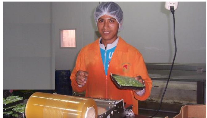
Fig. 6 Film sealing a 150-gram format - Snow Peas.
