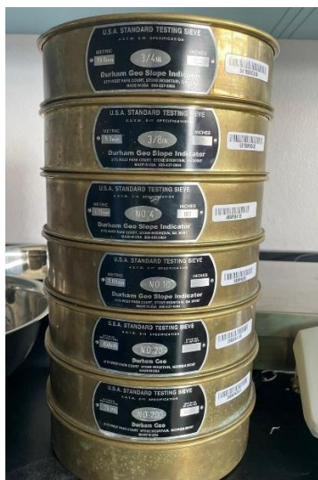
Figure 8. Tower of Sieves Used in the Aggregate Gradation
