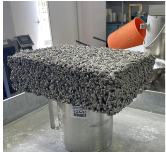
Figure.6. Pervious Concrete Slab
