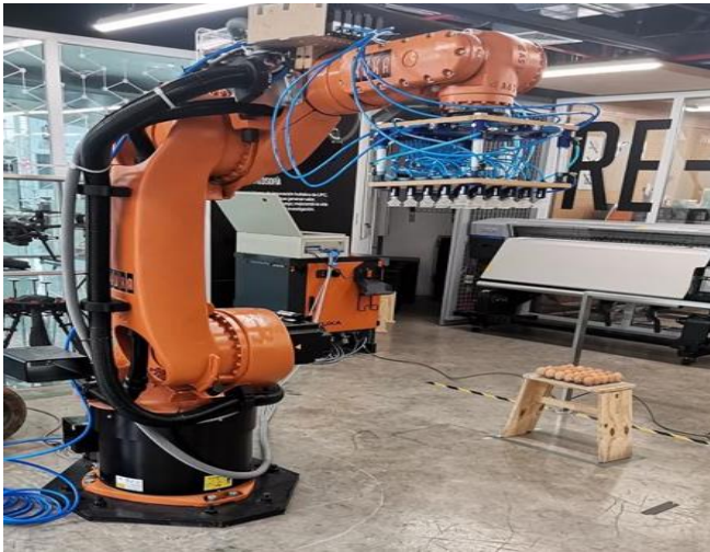
Fig. 9. Adaptable vacuum gripper final assembly.
