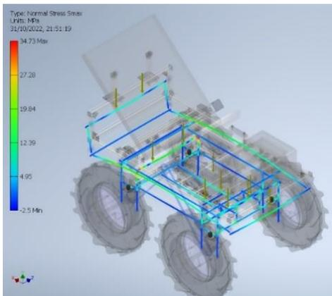
Fig. 7 Maximum normal stress on the chassis.
