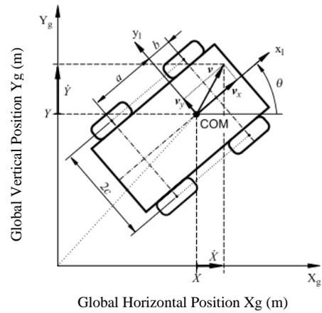
Fig. 6 Kinematic model [13].
