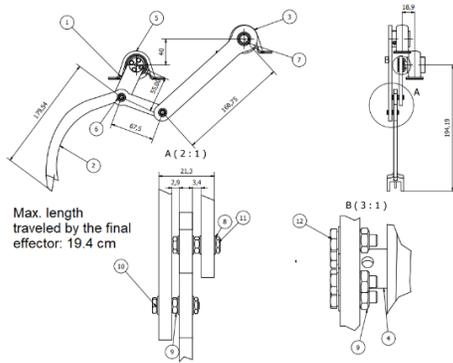
Fig. 3 Design of the transplant mechanism.
