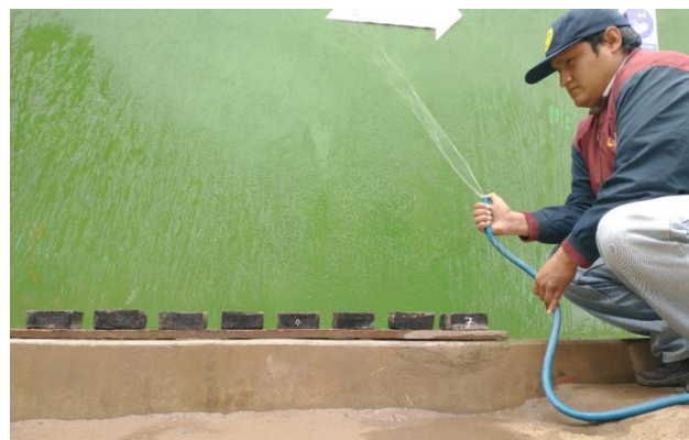
Fig. 8 Simulation of rain on samples subjected to exposure to polluting gases. Source: self-made
