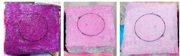
Fig. 5 Rhodamine B test - sample 7 (M-7), 0h, 4h and 26hr. Source: self-made
