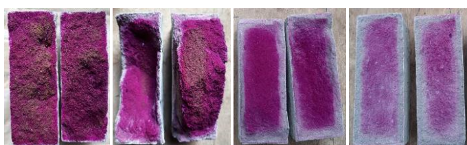
Figure 7 Reaction of mortar samples to phenolphthalein. Source: self-made
