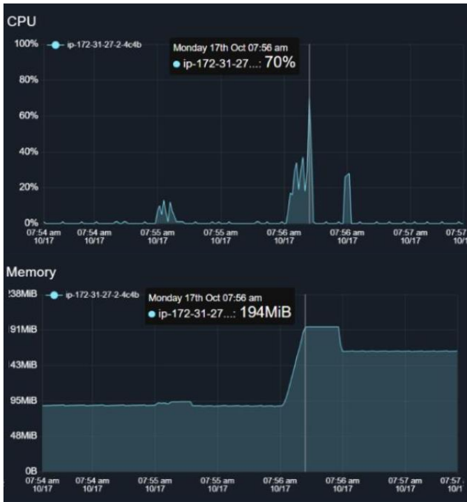
Fig. 16 “Download CSV functionality” CPU and RAM consumption on EC2.
