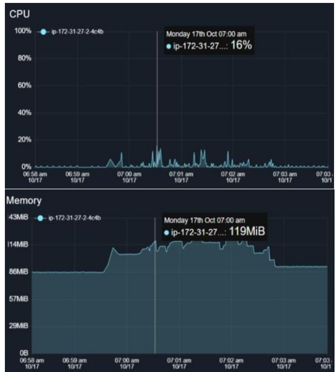
Fig. 15 JMeter CPU and RAM consumption on EC2 using pm2.
