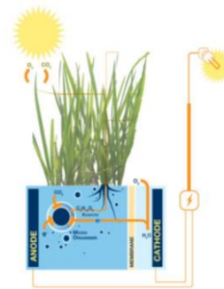
Fig. 3 Model of an electrical generation system based on a vegetable microbial fuel cell [38].
