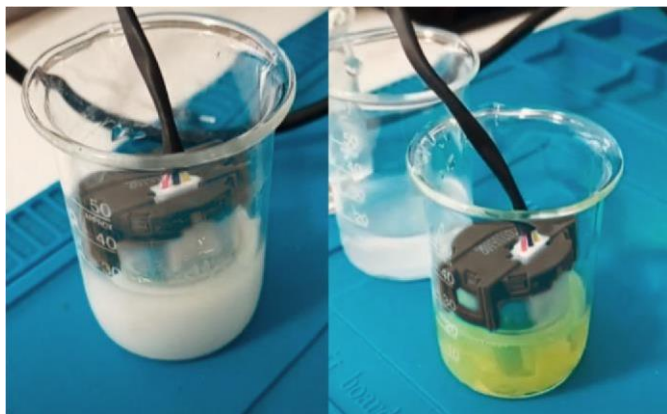
Fig. 9. Calibration of the turbidity sensor with different samples
