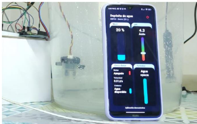
Fig. 11. Mobile application showing values measured by sensors.
