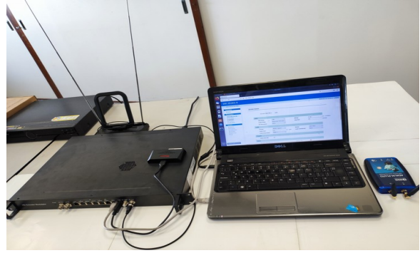
(a) PlutoSDR board used for the experimental evaluation. (b) Encoder and modulator to transmit television signals. Fig. 2 Hardware employed for spectrum sensing
